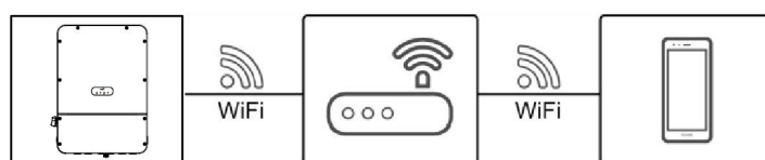
Figure 7-1 Mobile phone connecting to the hybrid inverter through a router
